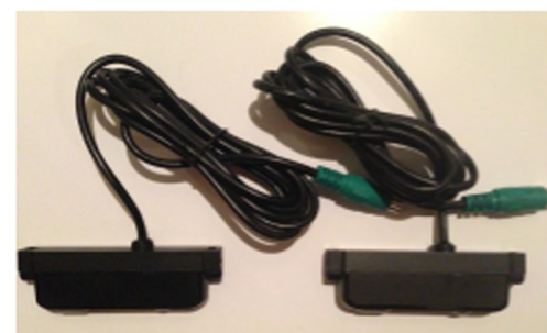
2 Laser Diffusers, mounted on front bumper of vehicle
