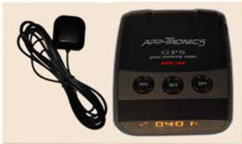
GPS 109 interior cab component GPS antenna
