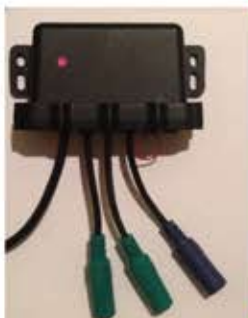
CPU/Wing Box-power supply for engine components
